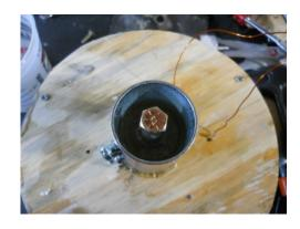
Step 22. Check the fit of the rotor to the stator and re-tighten the shaft nuts. Add as many washers as needed to adjust air-gap. 1/16" is a safe gap and still effective.
