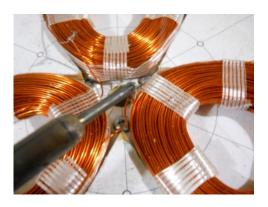
**Important:** Tuck all wiring as far away from the bearing tube as possible so that in a later step when you re-drill this hole there is no chance of cutting a wire.
