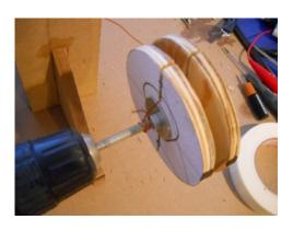
Step 10. Take a 6" length of magnet wire and pull through the slot and turn around the bolt a couple times.
