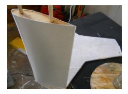
**Important** - keep the turbine square by measuring blade to blade, use a T square between blade and rotor.
