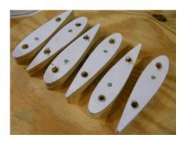
Step 6. Print out the blade former template and tack onto a double thick stack of 3/8" plywood. Put a #6 wood screw through each blade former between the 3/8" holes to hold the formers together as you cut the pairs out. First drill the 3/8" holes accurately or line up will be difficult and the blade may deform. Cut out 12 blade ribs.
