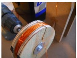
Unbolt the form and pull the coil off.
