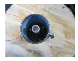
Mix up 2 oz of resin and carefully pour in. Do not fill past the level of the mid line on the coupler. Allow to cure thoroughly.
