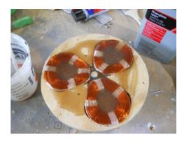
Lay the fiberglass cloth on and using a small brush saturate the cloth pushing down and around the coils.
