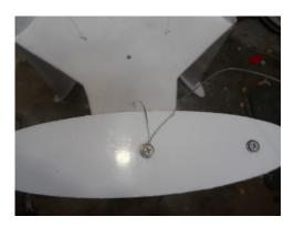
These tip should overhang at least ½" but not more than ¾". Any overhang at the leading edge causes
