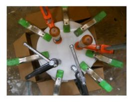
Make sure during the cure period the stator mold is on a level surface. Allow to cure for at least 4 hours. Go get a beer.
