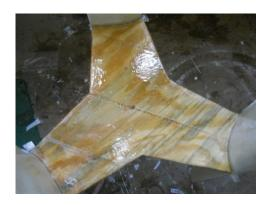
To paint fiberglass you first need to clean it. A good washing with soapy water, clean water rinse and drying.
