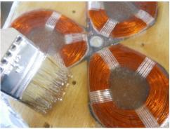
Lay a piece of polyethylene plastic on top (painter's drop cloth, kitchen trash bag etc..) on top. Put the stator press on and clamp down tight.
