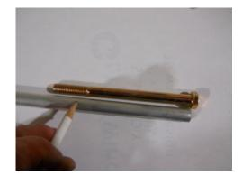
Cut off the head at ½" and grind the cut end smooth and with a slight bevel so that the turbine can easily drop into the bearing tube.
