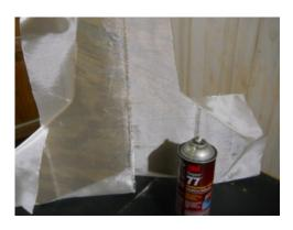
Spray the bottom of the rotor and pull the material over and trim in line with the rotor arms. Overlaps should be avoided. Trim along a straight line. Trim any loose bits until it all looks neat.
