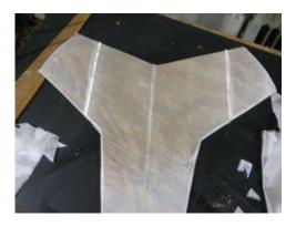
Step 2. Make slit cuts where the spar, shaft and bracing holes are in the rotor.
