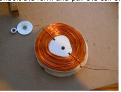
Take your strapping tape and tape around the coil legs at two places. Un wind the loose end wires and tape again at a third and fourth spot to retain the coil's shape.
