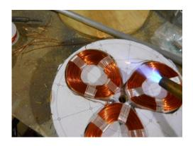
Take a start wire (inner wire) and an end wire (outer wire) from an adjacent coil and twist them together. Do this again with coil 2 & 3. **You must solder these joints.** Don't rely on just copper twisted. Tuck them in between coils towards the center where they wont contact any metal.
