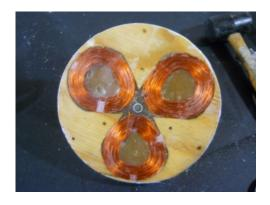
Remove the flash with some shears and a sander. **Caution:** Wear a respirator when sanding fiberglass. **Really!**
