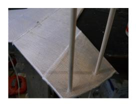
One way to keep things square is by placing the turbine on a drop cloth on the floor and square the top blades. The weight of the turbine will keep things straight while you resin the top sections. Let dry and turn over and resin.
